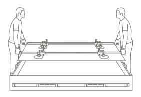
Handling the slabs on the floor can be managed with the aid of a frame fi ed with suction cups to make the slabs more stable.
