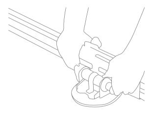
To facilitate handling of slabs with textured surfaces, the appropriate suction cups should be used.
