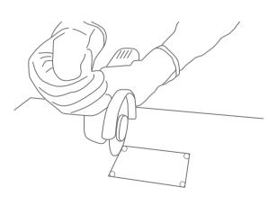
For L-shaped cuts or cuts inside the slab, holes should be bored at the vertices to prevent the blade of the cutting disk damaging the suface.
