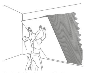
Once the slab is in position, access air should be removed completely by tapping it either manually or mechanically using the appropriate trowel, starting from the centre and moving out towards the sides.
