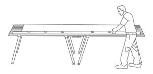
Cutting opeations should be carried out on a perfectly stable, flat surface.
