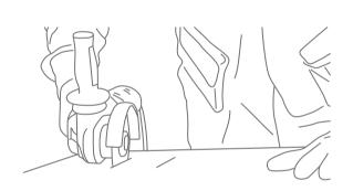
The slabs can also be cut with a dry saw or wet saw with a diamond wheel cuter.
