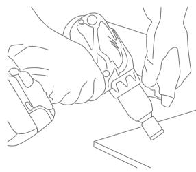
To bore cylindrical holes on the slabs, a diamond cutting ool of the desired diameter should be used, and the surface should be kept wet constantly.
